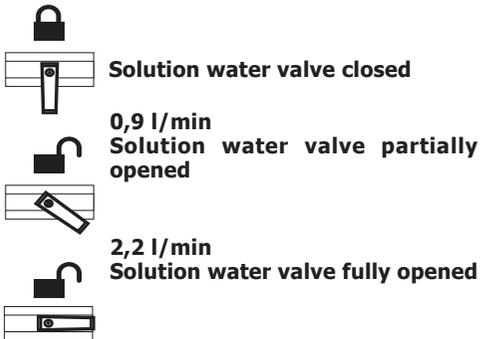
**Solution water valve closed**
