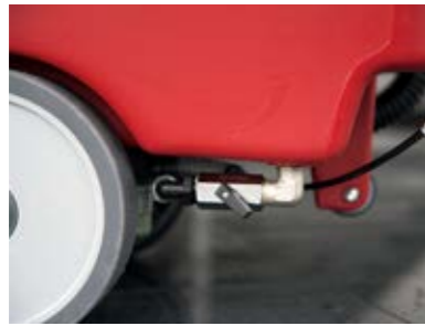
Water amounts can be adjusted individually to floor type.
