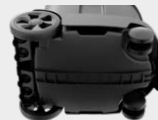
All-round elastic impact edges and a continuous sliding cam ensure a smooth transition over door thresholds.
