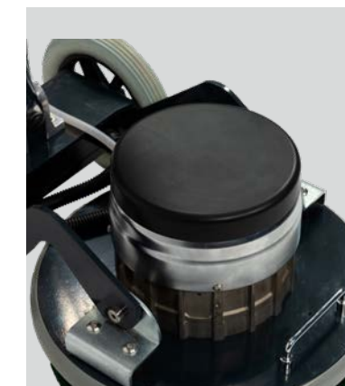
Motor protection cover protects the motor from moisture.
