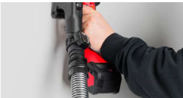
Activation via transmitter on the tool
